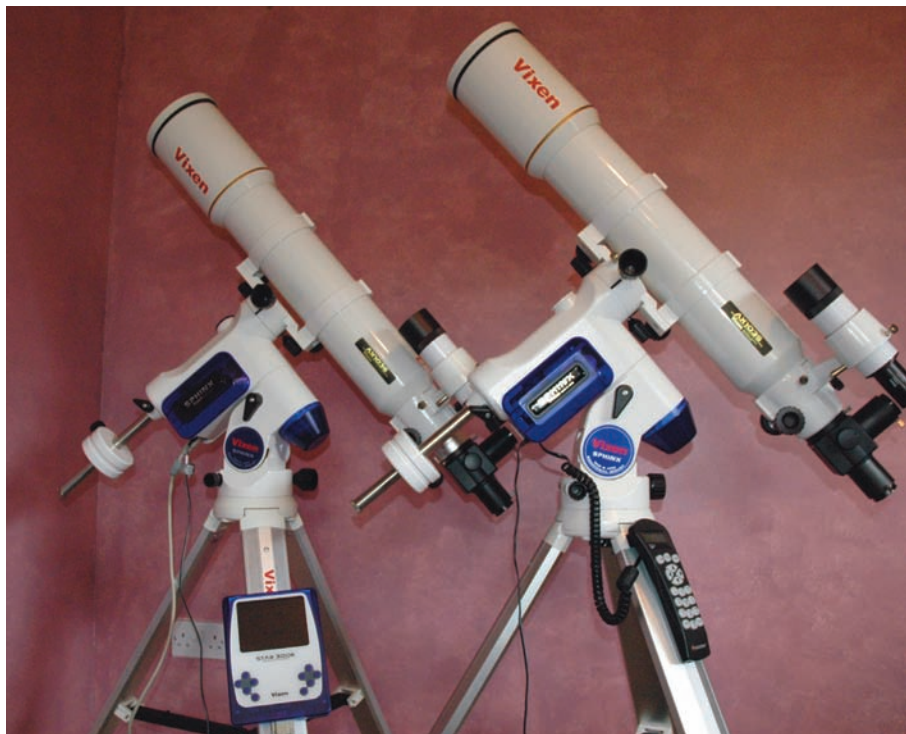
▲ The original Sphinx/Starbook system (left) next to the new Sphinx/NexSXD combination. All images: Ninian Boyle.
