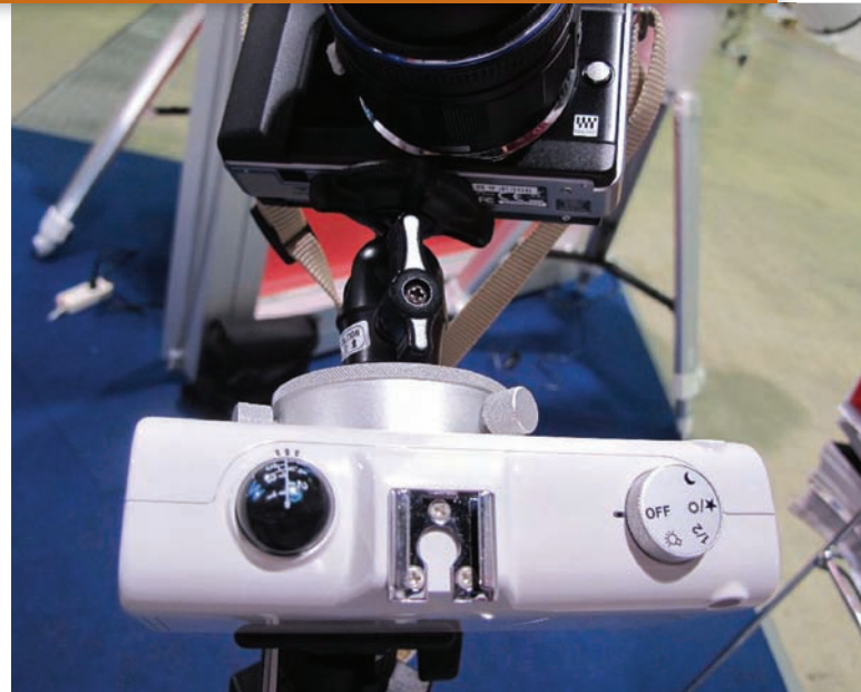
▲ A look at the controls on top of the Polarie, including the knob for altering the tracking rate – half and full sidereal rate, as well as lunar and solar. Image: Pete Gamby/Vixen.
